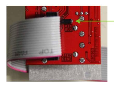
To enable your drum modules for Bus Mix look for the header located on the back of each module and place the header on both pins. You can enable some and disable others to decide which ones you want to be mixed by the MIXZ. Remember, you can always add them later to the mix through the front panel Mixer A and B.
