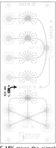
mixer. It has gain control for each channel. The out internally routed to Mixer B. If you plug a patch cable into the out it will break the connection to Mixer B so Mixer A can be used independently from Mixer
